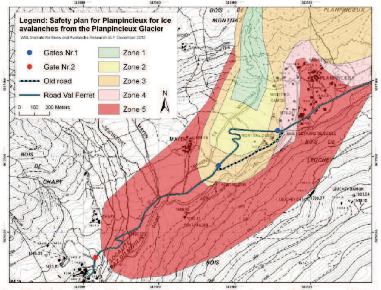
Fig. 22: Safety plan for Planpinceux for ice avalanches from the Planpinceux Glacier (Important remark: the area is also endangered by snow avalanches from other release areas. These avalanches are not considered in the safety plan!).
